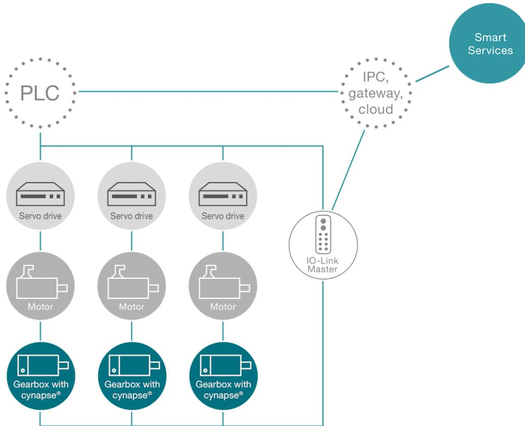
Using this system as an example, the gearboxes with cynapse® are connected to an IPC/gateway via an IO-Link master in addition to the PLC via a separate network connection. This IPC serves as a Docker host and offers the option of integrating additional machine data from the PLC or sending data to the cloud using WITTENSTEIN's Smart Services.
