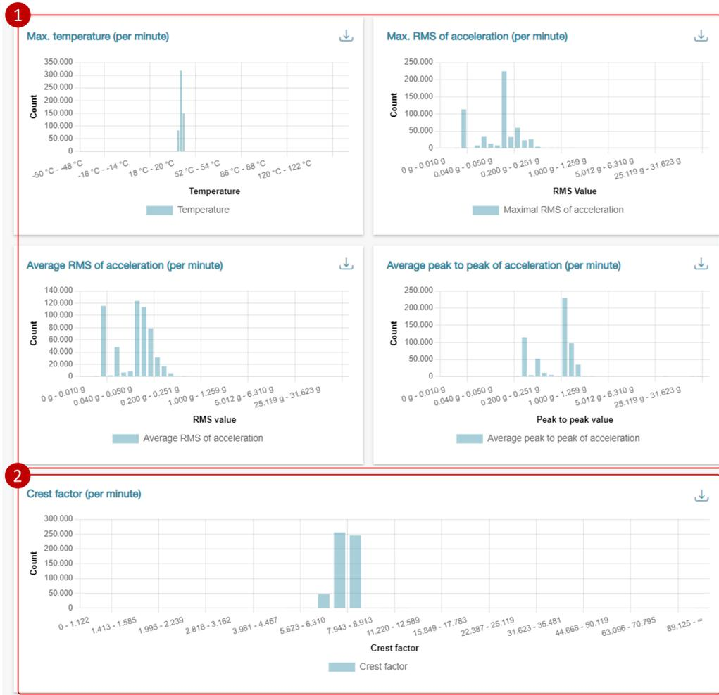
Besides visualization, cynapse<sup>®</sup> Monitor supports the export of individual histograms. Each histogram has an export button which can be used to initiate the export. When pressed, a CSV file containing the histogram labels and data is generated and downloaded to your computer.
